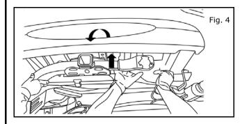
6) Rotate hitch into position with the help of an assistant.
